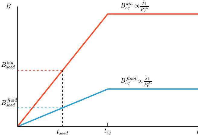
FIG. 2. Schematic picture of the magnetic field growth. Magnetic field grows approximately linearly with time until it saturates at equilibrium value  $B_{eq}$ . Kinetic effects increase  $B_{eq}$  to the same extent as they increase the current drive efficiency, but they hardly change the time to reach equilibrium  $t_{eq}$ . The actual value of the magnetic seed is determined at some characteristic time  $t_{seed} \ll t_{eq}$ , and it increases to the same extent as the efficiency increases.
