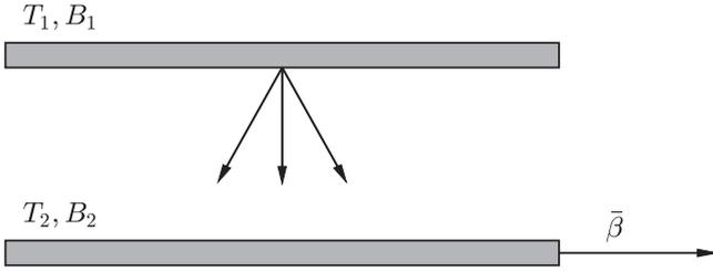
FIG. 1. Parallel radiating and absorbing slabs of plasma, immersed in different magnetic fields at different temperatures, in relative parallel motion.
