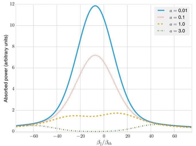
FIG. 4. Absorbed power density per electron as a function of parallel velocity for  $\beta_{th} = 0.01$ ,  $\bar{\beta} = 0.05$  and different values of  $a$ :  $a = 0.01$  (solid blue),  $a = 0.1$  (dotted red),  $a = 1.0$  (dashed orange),  $a = 3.0$  (dash-dotted green).
